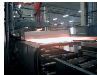
SSAB - Sweden Glue preheating
