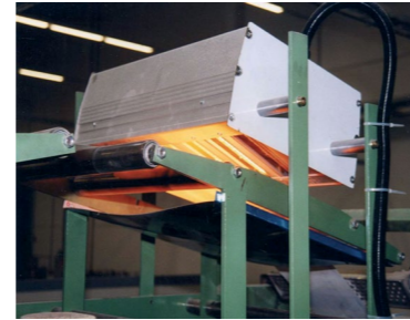
Hantermann - Germany Ink drying on napkins in a flexo printing machine
